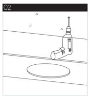
Drill the upper ceiling Ø12 for anchor bolts -RB380.002.CR: 3holes for triangle(three sides 280mm) -RB430.002.CR: 4holes for squ are(260 mm)
